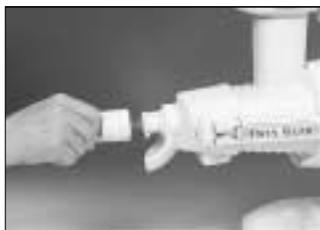
2. Turn the **Outlet Adjusting Knob** counter clockwise until it separates from its threads; then pull it out from its grooves.
